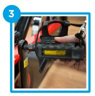
Make sure the pedals are aligned straight to the crank
